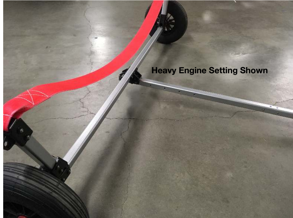
Adjust Axle Location on Aft Tongue Tube based on boat length and other load variables like the engine. Move it farther back for a heavier engine and farther forward for a light engine or no engine. The goal is to achieve a handle weight of 20lbs or less. Small changes can make a big difference!
