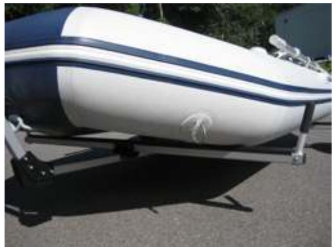
**Type 10 Dolly** — This sling-less dolly works well on smaller inflatables, especially those with a flat, soft bottom or those with a high pressure keel. The cross bars that the boat rests on are covered in a durable, non-marking, vinyl rub rail.
