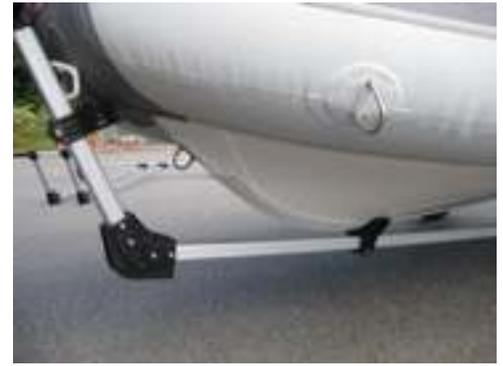
**Type 1 Dolly** — This single tongue, single axle dolly is ideal for hard bottom or high pressure keels. Our rugged “V-Fitting” cradles the keel of the boat. Eyelets on the bow and side tubes provide a convenient tie down point.
