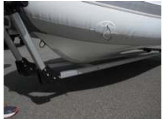
**Type 5 Dolly** — This double tongue, single axle dolly works well for larger hard bottom boats. The boat's keel rests on a “keel tube” that links the dolly tongues together. The keel tube is covered in a braided hose.
