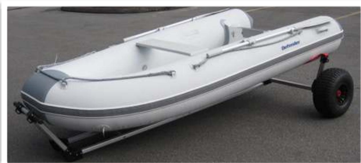
The variety of design and size of small inflatables makes for a challenge when picking the “right” dolly for your boat. Dynamic offers several types of dollies that help satisfy the wide range of inflatables. Two wheel sizes, Standard or Large, allow users to choose the tire that works for the terrain they encounter (Large Wheels Above). Delrin® ball bearings make for an effortless roll. Dynamic Dollies are designed to last in the harshest environments with little maintenance.
